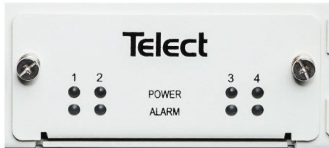
Fig. 11: Replacing the alarm card
