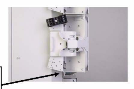
NOTE: When proper installation is achieved, there should be no space between the module and the main frame as pictured here
