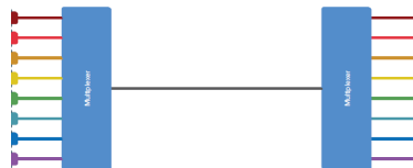
Fig. One strand of single mode fiber can carry many different modulated signals using WDM
