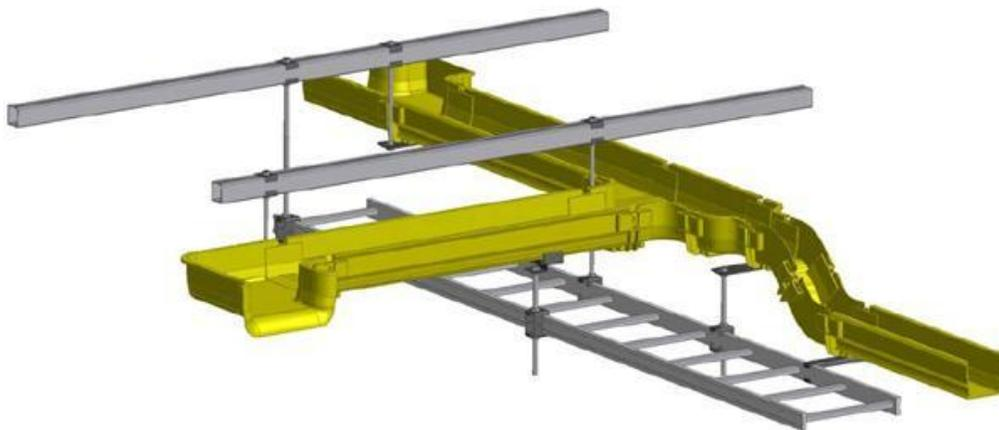
Fig. 2-2: Trough support system
