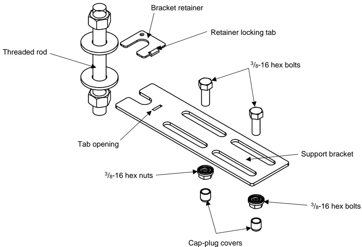
Fig. 2-4: Threaded rod bracket
