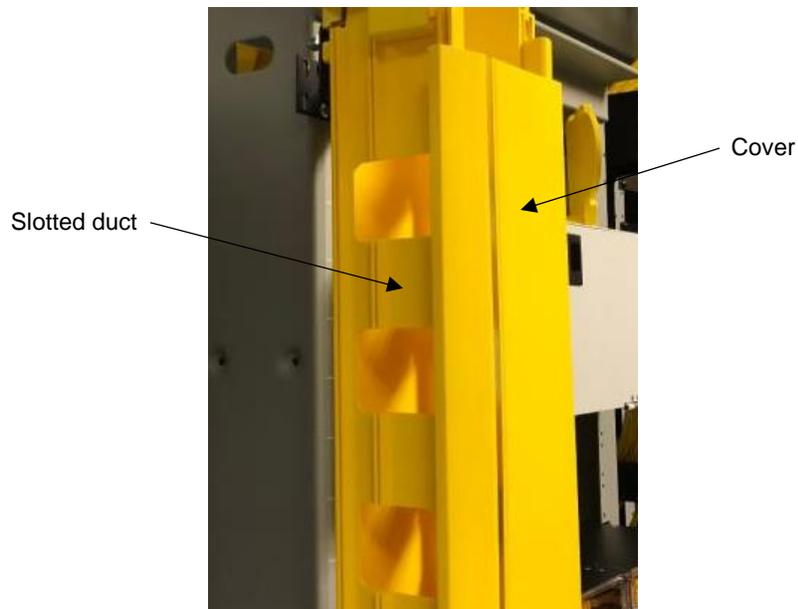
Fig. 4-65: Installing the slotted duct cover
