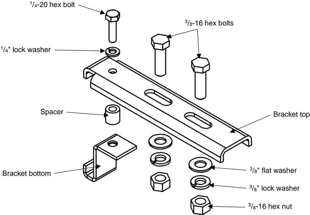
Fig. 2-11: Cable rack bracket
