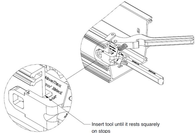
Fig. 3-2: 24" Notching Tool guide
