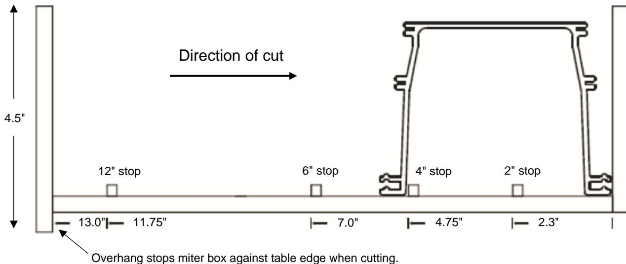
Fig. 3-0: Custom miter box drawing
