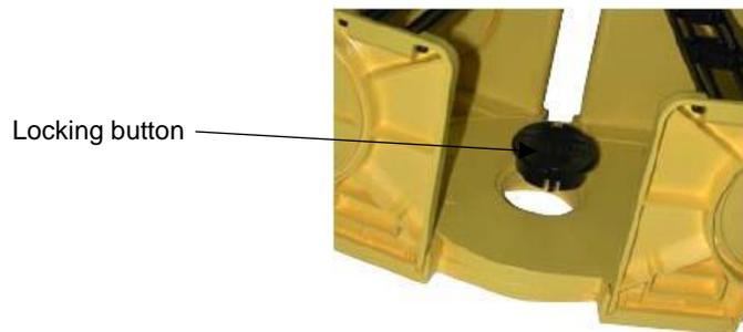
Fig. 4-22: Locking 6" CableLinks together
