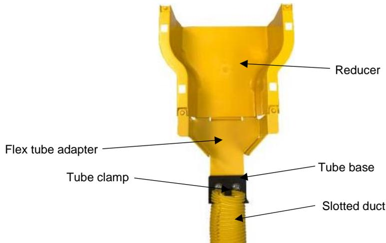
Fig. 4-70: Connecting split tube to the tube clamp
