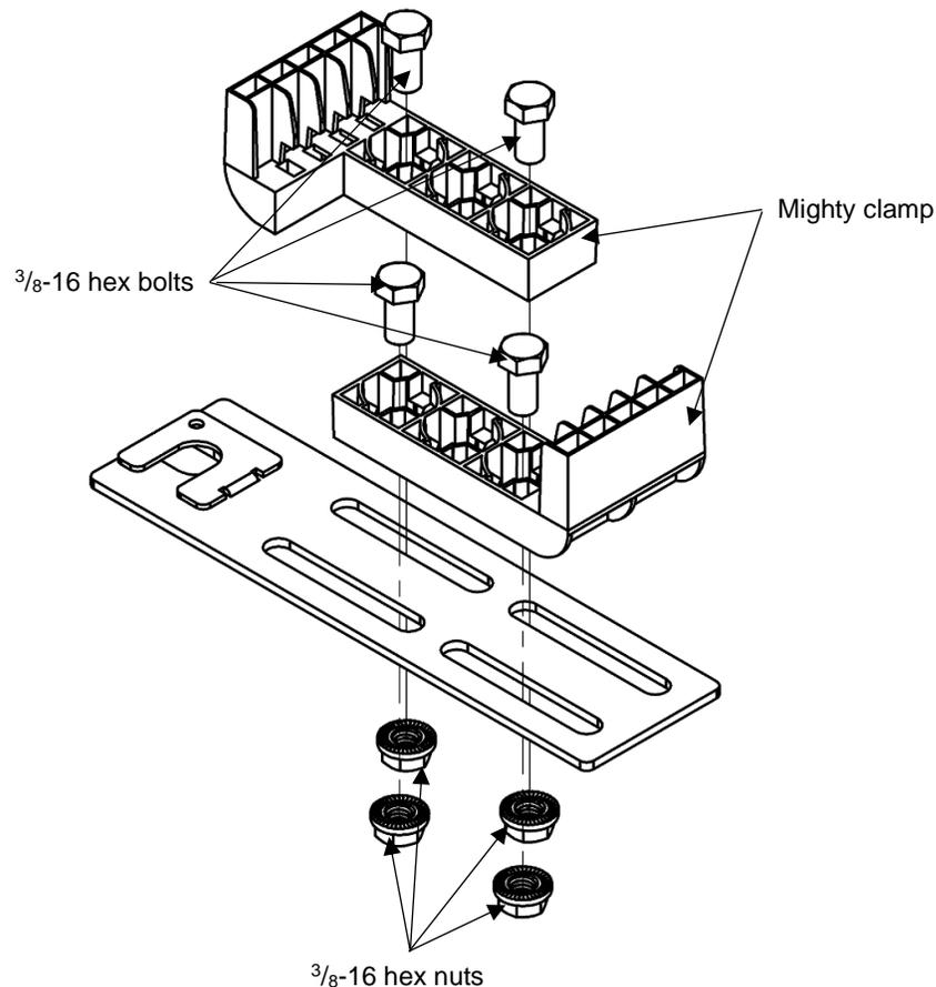
Fig. 2-7: Trough support clamp (mighty clamp)
