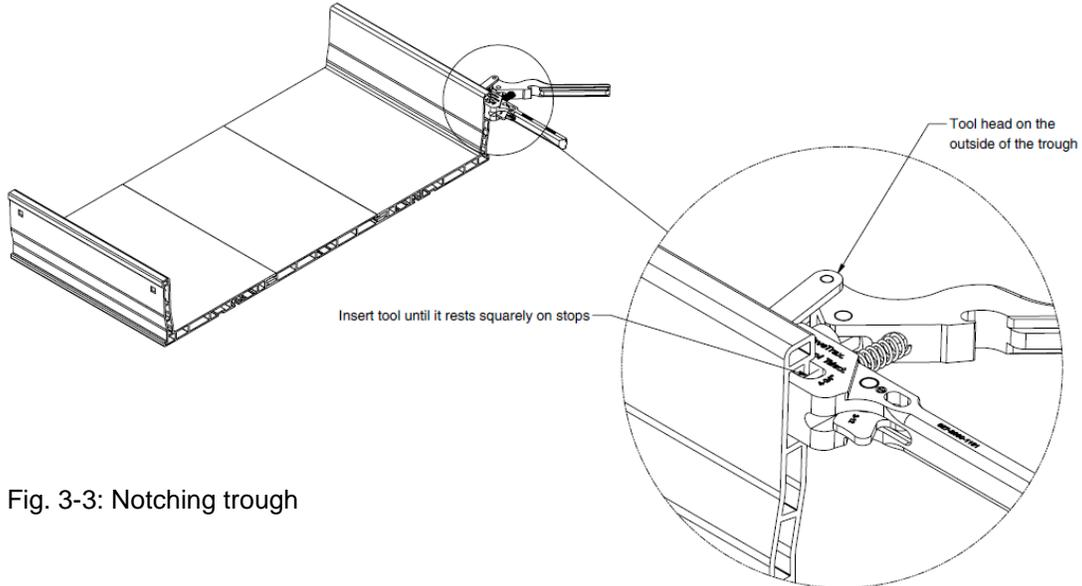
Fig. 3-3: Notching trough
