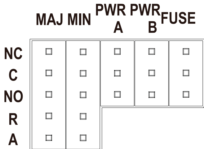
Figure 7 - Alarm Terminals on all panels except HPGTM10FA-1RU
